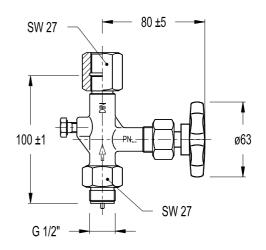
DESCRIPTION Gauge coil for pressure gauge. MAIN FEATURES Complete stainless steel AVAILABLE MODELS: GSC-40 CONNECTIONS : DN ½" (male x female) PMA Max. allowable pressure :40 bar
