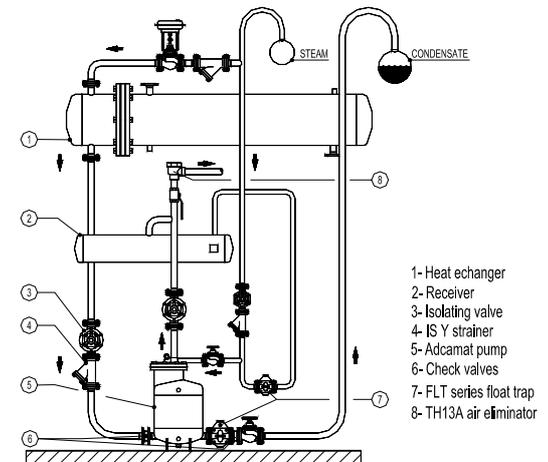
**Drainage of a single unit under vacuum**
