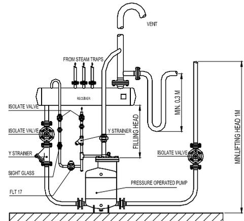
Removal of condensate under pressure with POP pump and steam trap combination. When the steam pressure is sufficient to overcome back pressure the trap operates.
