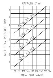
Example: We require to inject 950 Kg/hr of steam with a pressure of 5 bar. Assuming 20% pressure drop across the control valve, therefore the steam supply to the injectors will be 4 bar. From the injector capacity chart we see that the 4 bar injector will pass 293 Kg/hr and 950 divided by 293=3,24.
