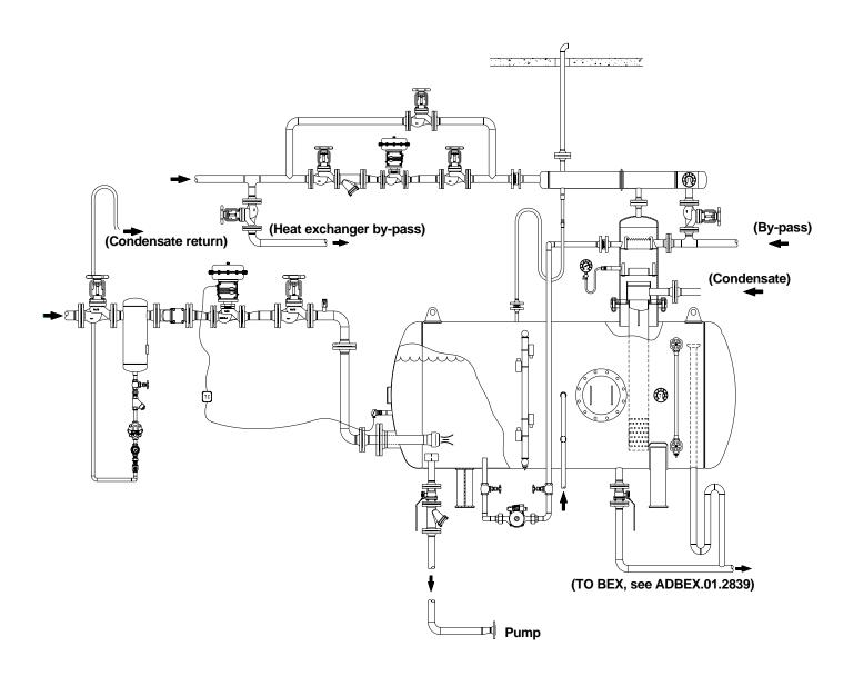
Atmospheric deaerator including Adcatherm-STS series complete stainless steel heat exchanger. Make up water crossing the heat exchanger will condense the flash steam, preventing energy waste and better performance of the whole system.
