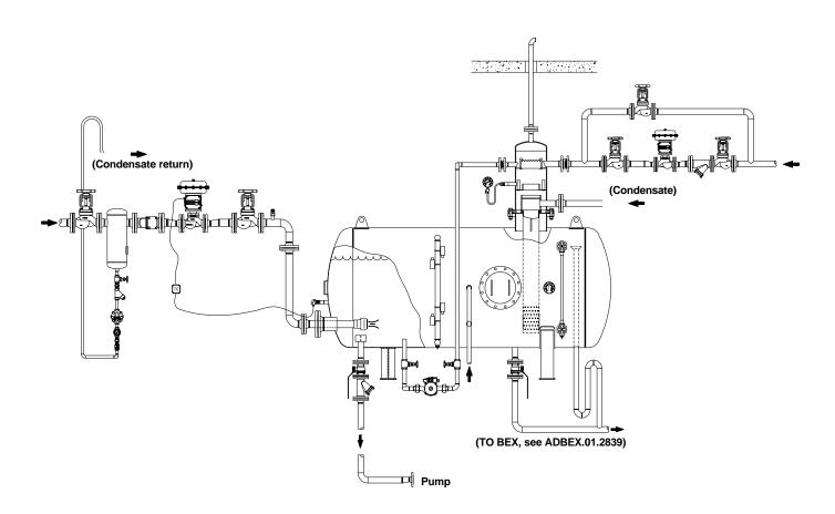
Atmospheric deaerator provides an economical system to preheat boiler feed water and drive off dissolved gasses.
