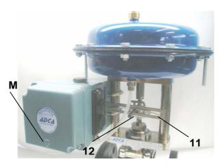
Ensure that the feedback lever **11** is horizontal at 50 % stroke.
